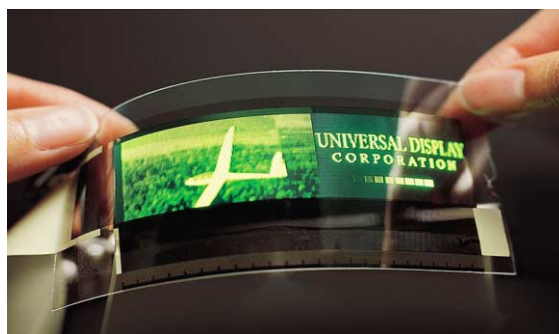
Fig. 10. A video rate 240 × 64 80 dpi passive matrix monochrome green PHOLED display fabricated on a barrier-coated 175-μm-thick PET substrate.
